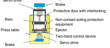
**In general:** If a gating of the safety system respectively an acceptance of the control command is realized during the opening stroke, a pendulum stroke must be avoided (change of the direction outside normal operating conditions). The safety distance has to be determined before the startup by a follow-up movement.
