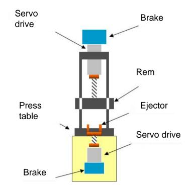
Servo presses are mechanical presses which have a power transmission <u>without mechanical clutch</u>. At this kind of presses the mechanical clutch is replaced by the power transmission of a servo drive (electric motor with control device). If a safe switch-off (stop) of the servo drive is realized the pestle is kept in position by means of a safety-related brake.
