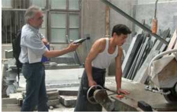
Gerhard Czuck, Germany, measuring the noise level at the work place
