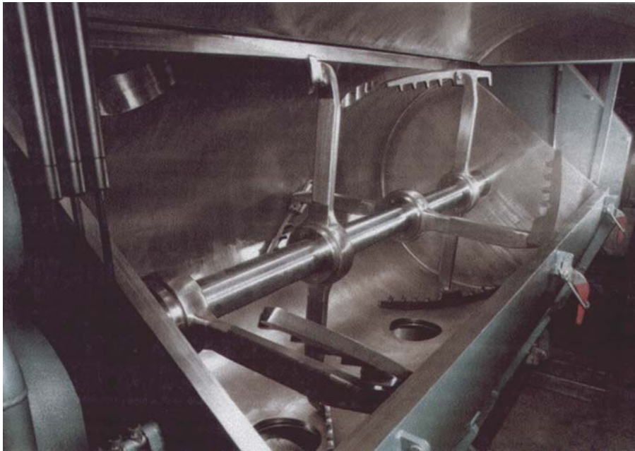
Fig. 19: Schematic presentation of a horizontal mixer (top). View into an opened horizontal mixer (left). [Picture: Prof. Dr-Ing. Drs h.c. Manfred H. Pahl, University of Paderborn]
