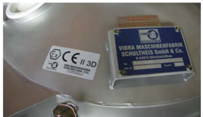
Fig. 23: Vibro screener (left). Right: Detail of earthing and tag plate which indicates that the screener is category 3D (externally).
