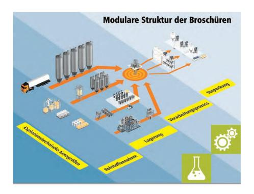
In the process step "storage", flammable and dust-explosive bulk materials are stored in halls, bunkers and containers. Silos made of metals, concrete, plastics or flexible fabrics are also used. If nothing to the contrary is noted, it is assumed that the bulk material is free of flammable solvents and that the environment of the product is free of flammable gases and vapours (see module: safety characteristics).
