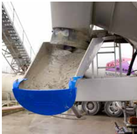
Keeping roads clear of concrete spills and drivers safe: the cover engineered by Michael Gräbe of streeprotec.
