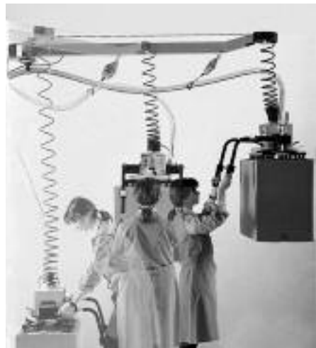
Figure 8: Moving of loads with a vacuum lifting device
