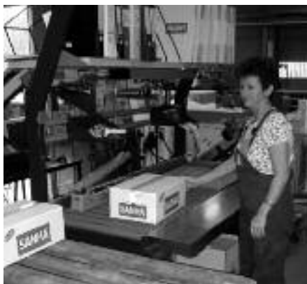
Figure 10: Prevention of lifting and carrying activities through vertically adjustable work tables and roller conveyors
